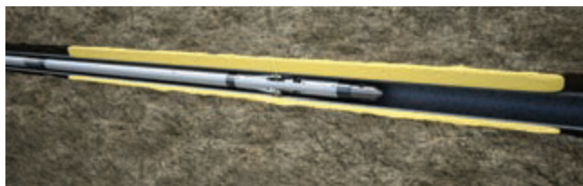
Fig. 1—Injected sealant forms an annular isolation barrier. Images courtesy of CannSeal.
